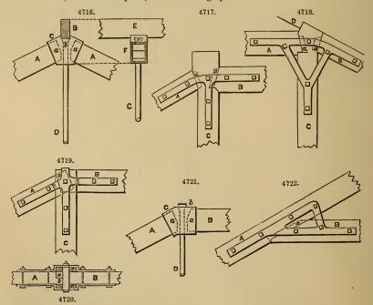
Figs. 4717 to 4721 illustrate the mode of framing together the principal rafter, queen-post, and straining-piece. In the first three examples the joints are secured by straps and bolts, and in the
